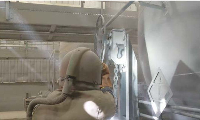
KinetiX 20/70 removing tough, high solids epoxy from a rail car
