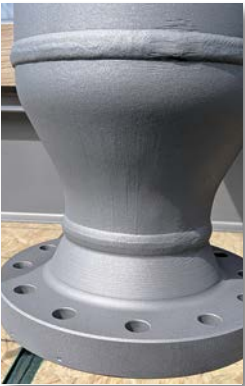
Background photo: close-up of this pipe flange surface, blasted with 10X abrasive. Note the quality of finish on welded area.
