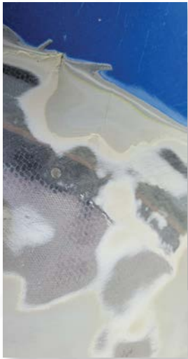
EpiX MP removing urethane-based coating from Pilatus PC-12 composite aircraft engine cowling without causing damage
