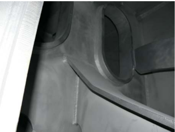
Day 3, after blasting with KinetiX: graded SSPC-SP5 clean white metal finish
