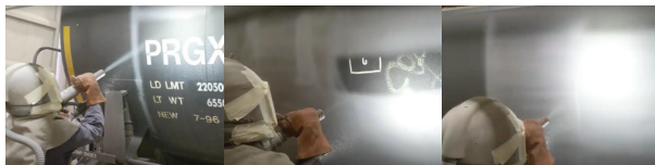
The test process compared performance in exterior refinishing of tank cars using olivine vs. 10X superoxalloy abrasives at 110 psi pressure using Kennametal XL #10 nozzles.
